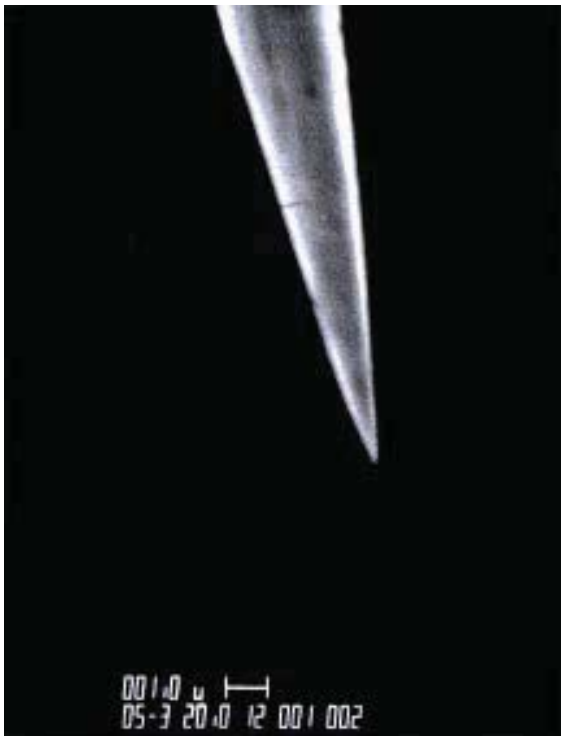
Scanning electron microscope photograph of a T-4-10 Tungsten point. (1 micron = 0.5 cm)
